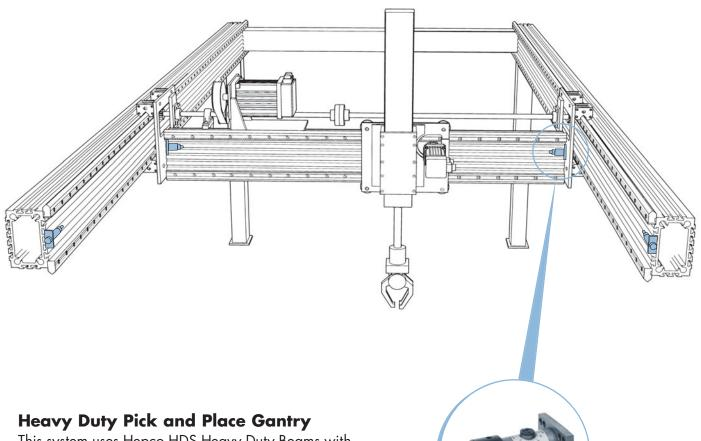
This system uses Hepco HDS Heavy Duty Beams with Single Edge Slides and rack drive on the X and Y axes. Shock Absorbers are used here as a safety protection feature in case of limit switch failure causing motor over-run.
