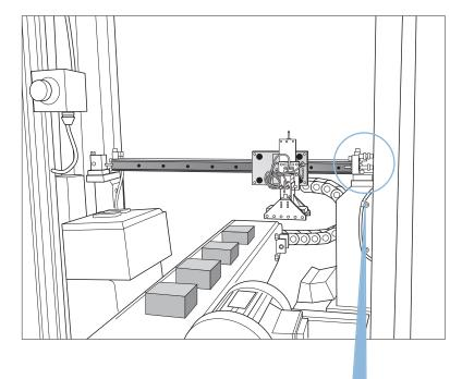
horizontal slide by a friction drive.
